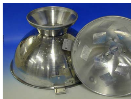
Figure I. Scheme of the Wheeler cap method and some of the Wheeler caps used in the measurements.
